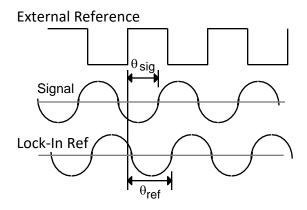
The lock-in amplifies the input signal and then multiplies it by the reference signal using a phase-sensitive detector (PSD) or multiplier. The output of the PSD is simply the product of two sine waves.
